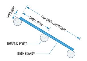
These Span Tables were developed using No. 2 & better grade lumber using WWPA grade rules as an industry standard. Higher or lower grades are available, impacting the span values.
